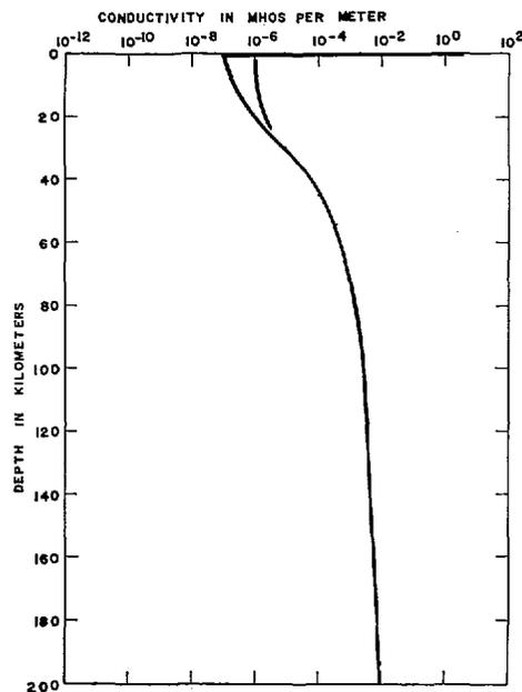
Fig. 3—Electrical conductivity below the sea bottom.
