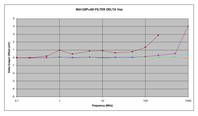
Figure 10-5. Input Offset Shift With Analog Devices' Filter: Note  $\pm$  5mV Vertical Scale.
