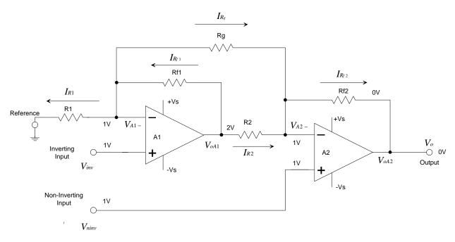
Figure 3-7. Two Op Amp IA Common Mode Rejection Analysis.
