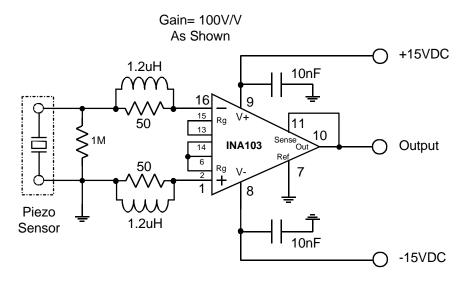
Figure 4-1. An Unsuitable IA Choice For A High Impedance Transducer.
