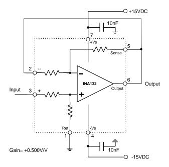
Figure 6-5. A Precision Gain Of +0.500V/V.
