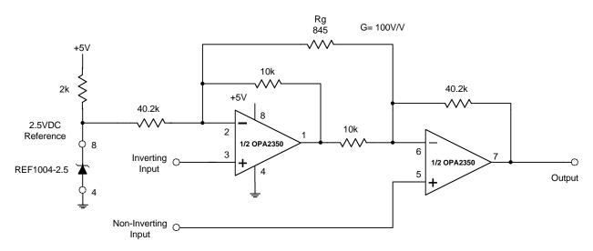
Figure 8-1. A Fast R-R Single + 5V Supply Instrumentation Amplifier With A Gain Of 100V/V.
