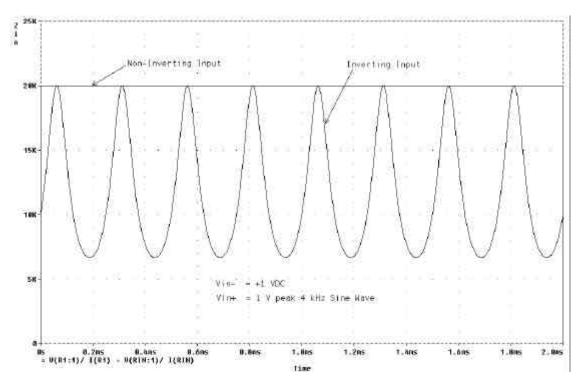
Figure 6-10. Unexpected Behavior? Difference Amplifier Inputs Exhibit "Different" Loading Of Their Respective Signal Sources.
