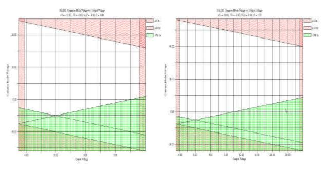
Figure 9-7. (a.) INA132 Common Mode Range With + 12/-5VDC Supply (b.) INA132 Common Mode Range With + 28/-5VDC Supply
