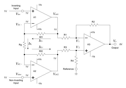
Figure 3-4. Three Op Amp IA Common Mode Voltage Analysis
