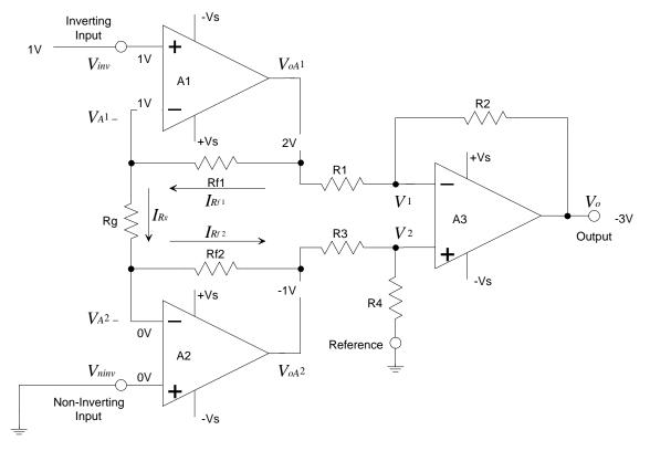
Figure 3-3. Three Op Amp Instrumentation Amplifier Gain Analysis
