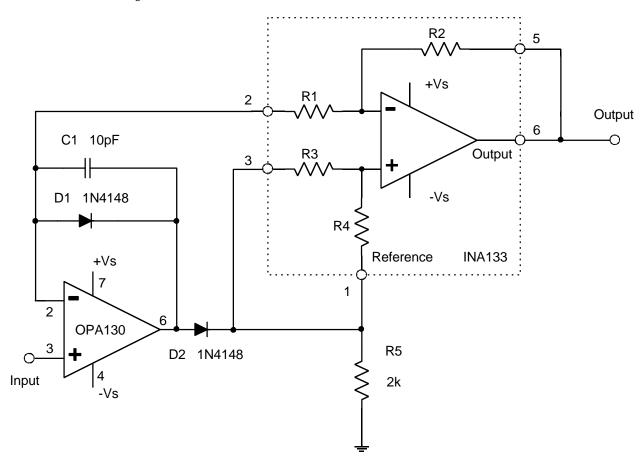
Figure 11-1. Unity Gain Absolute Value Circuit- Positive Output.
