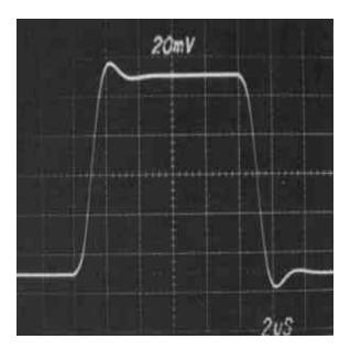
Figure 6-2. Even With The 0PA27 Op Amp feedback circuit gain of 0.5V/V and 1000pF load, the stability of the INA117 circuit is excellent
