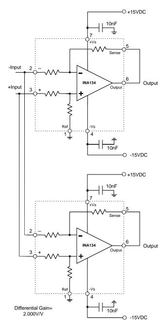
Figure 6-6. A Differential- Input/ Differential- Output Amplifier.
