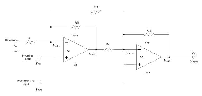
Figure 3- 5. The Two Op Amp Instrumentation Amplifier
