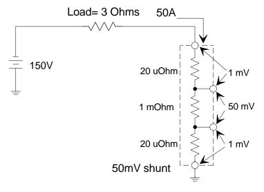
Figure 7-2. Shunt Resistor Kelvin Connection
