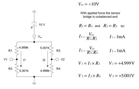
Figure 2-4. Unbalanced Bridge Generates A Differential Output Voltage.
