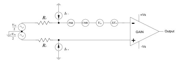
Figure 2-5. A Model Of Input-Referred Errors.
