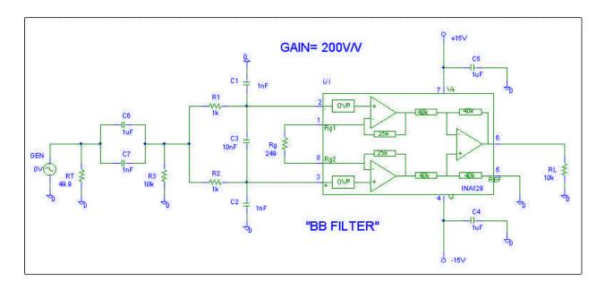
Figure 10-9. RFI Test Circuits For Measuring Offset Shift Of INA129 With "BB" LPF.
