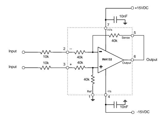
Figure 12-1. How To Ruin Your Difference Amplifier's Common Mode Rejection- Add External Resistors.
