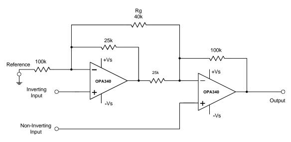
Figure 9-8. A R-R Input And R-R Output Instrumentation Amplifier With a Gain Of 10V/V.
