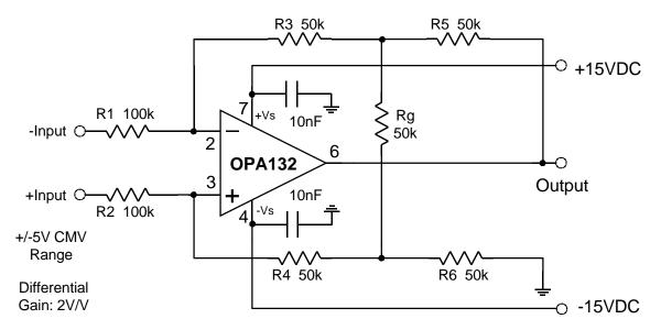
Figure & 4. A "Different" Resistor Network Plus An Op Amp Yields An Adjustable- Gain Difference Amplifier
