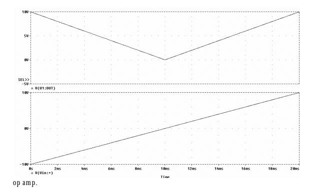
Figure 11-2. Absolute-Value Circuit Input (Bottom Curve) vs. Output (Top Curve) Transfer Function. The Amplifier's Output Is Always Positive.
