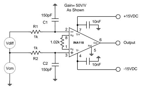
Figure 4-15. Noise and RFI Filtering- The Wrong Way.
