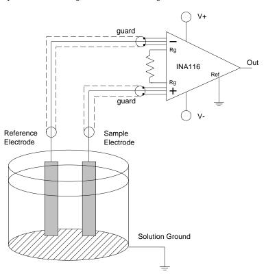
Figure 9-1. Amplifier For pH Measurement
