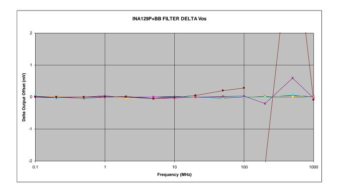
Figure 10-7. Input Offset Shift With Improved "BB Filter": Note  $\pm$  2mV Vertical Scale.
