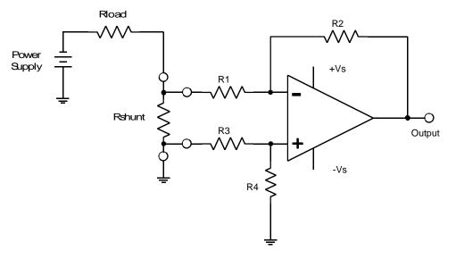
Figure 7-3. Differential Sensing Of The Voltage Drop Across A Low-Side Shunt Resistor Minimizes Ground Loop Errors
