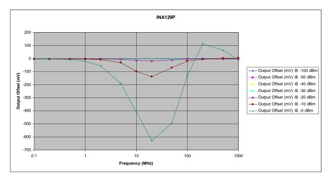
Figure 10-2. Unfiltered INA129 Input Offset Shift: Note +200, -700 mV Vertical Scale.
