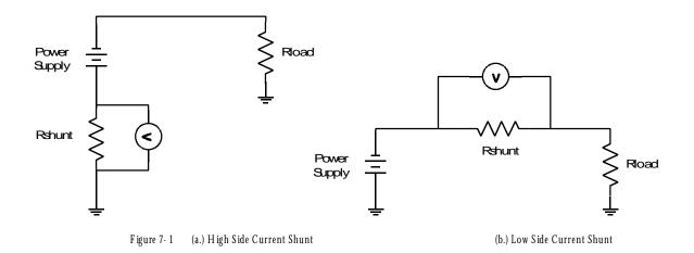
Often, there may be shunts on multiple supply outputs so that current can be monitored into each circuit branch. This necessitates a high side shunt convention. A low side shunt placed in the power supply ground return in this example would measure the total supply output current.
