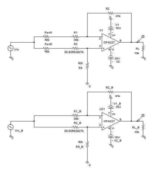
Figure 12-2. Circuit Diagram To Investigate Effects Of Adding External Resistors To A Ratio-Trimmed Difference Amplifier.
