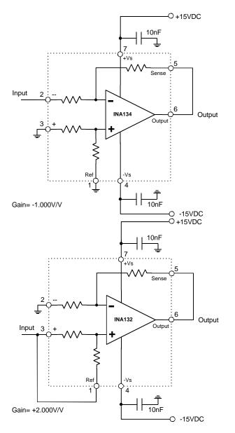
Figure 6-3. (a.) Precision Gain Of -1.000V/V Amplifier.
