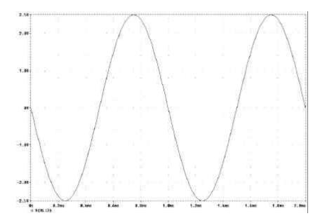
Figure 9-9. OPA340 Instrumentation Amplifier R-R Output Swing Into A 10k Load With Vs =  $\pm 2.5$ VDC And Vin = 250mV p.p.
