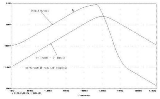
Figure 4-19. CMV Frequency Response of INA118 Instrumentation Amplifier with Mismatched Common Mode Low Pass Filter Poles.
