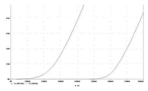
Figure 10-1. I-V Curves For Germanium and Silicon Diodes.
