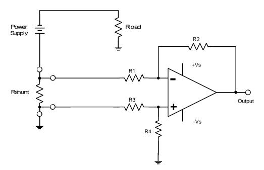
Figure 7-4. Alternative Connection Of Shunt Resistor. Re: Figure 24.
