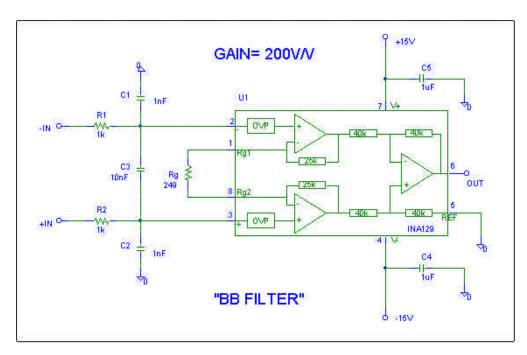
Figure 10-6. An Improved All Passive Input Filter-Dubbed the "BB Filter."
