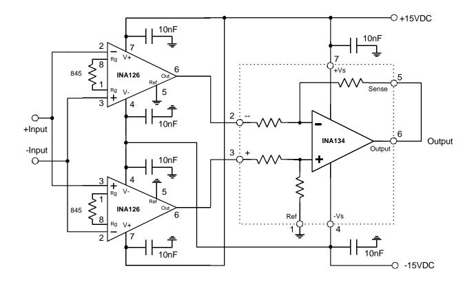
Figure 9-4. "Mirror Image" Amplifier Extends High Frequency CMR Of Two Op Amp Instrumentation Amplifiers.
