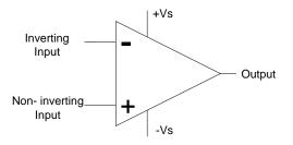
Figure 2-1. A "Black Box" Representation of an Instrumentation Amplifier.
