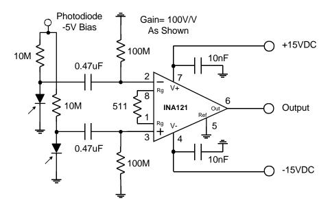
Figure 4-5. Adding Bias Current Return Resistors Solve The Problem.
