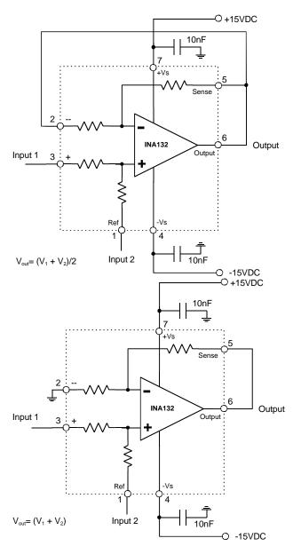
Figure 6-4. A Difference Amplifier Connected As (a.) An Average Value Amplifier. (b.) A 2- Input Summing Amplifier.
