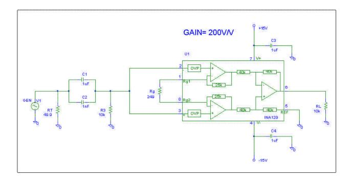
Figure 10-3. Unfiltered Input INA129 RFI Test Circuit.
