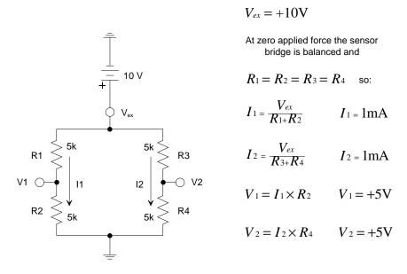
Figure 2-3. Balanced Bridge Generates CMV But No Differential Output Voltage.
