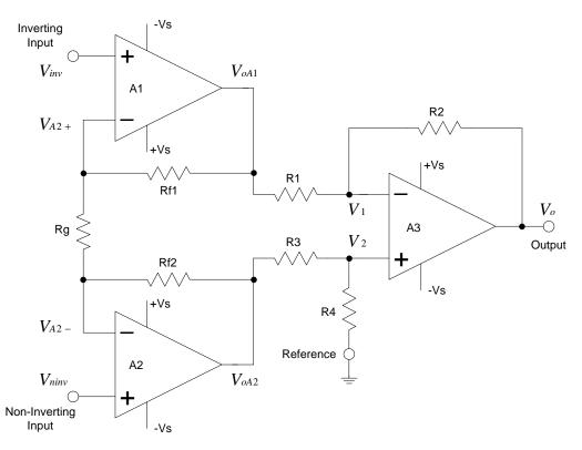
Figure 3-2. The "Classical" Three Op Amp Instrumentation Amplifier.
