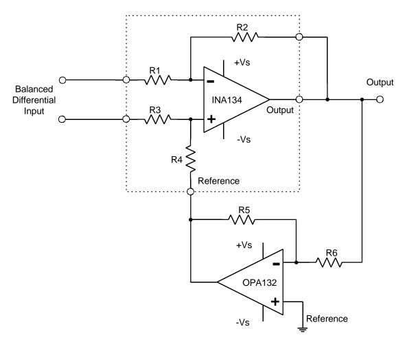
Figure 6-11. Is The Input Loading of This Circuit Better Than Figure 6-10?
