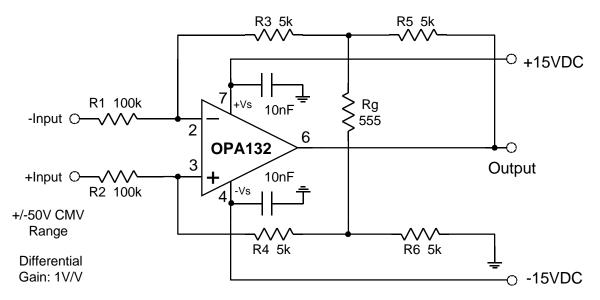
Figure 8-5. Adding Gain To Compensate For An Input Voltage Divider Yields A Unity Gain Difference Amplifier With A 50V Common Mode Voltage Range.
