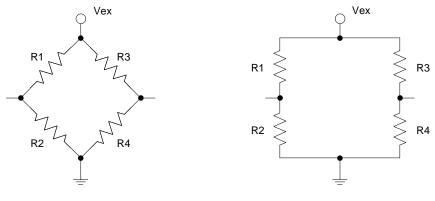
Figure 2-2. (a.) Conventional Bridge Circuit.
