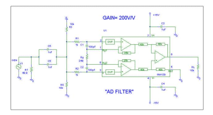
Figure 10-8. RFI Test Circuits For Measuring Offset Shift Of INA129 With "AD" LPF.
