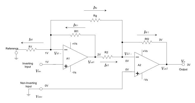
Figure 3- 6. Two Op Amp Instrumentation Amplifier Gain Analysis.
