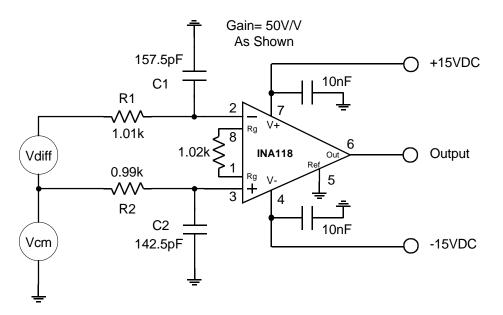
Figure 4-16. Worst-Case Mismatched Pole RFI Filters With 1% Resistors and 5% Capacitors.
