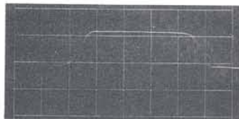
Fig. 1. The accompanying photograph shows the pulse response of the Type 517 Vertical Amplifier. The sweep rate is 10. \text{m}\mu\text{sec}/\text{cm} . Note rise-time and freedom from ringing and overshoot.
