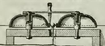
by the bells. The patent also describes a novel spiral spring gong, a pair of which can be made adjustable in a similar manner to that described for ordinary bell gongs. For the gongs here illustrated, there is provided a pair of sound dampers, or modulators, consisting of small thin pieces of fiber, felt, celluloid, or other suitable material, which are securely fixed in a specific manner to the outer edge of the bells.
