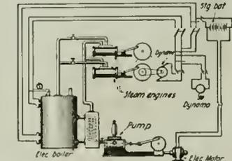
switched on to an electric motor connected with a pump for supplying fresh cold water to the boiler, this water being pre-heated by means of the exhaust steam coming from the steam engines shown. Thus the electric circuits and steam generating apparatus work hand in hand apparently, without any energy from an outside source of electric power being supplied to the electric boiler circuits, except from a small dynamo at "starting."
