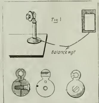
happily subject to. The present design provides a non-twisting balance weight which may be attached to or detached from a 'phone cord instantly, without in any way mutilating the cord, and also, without having to disconnect the telephone instrument from the cord. The inventor claims that his device solves the problem correctly, by virtue of the fact that the weight is fixed to the cord upon a different center than that of the cord.
