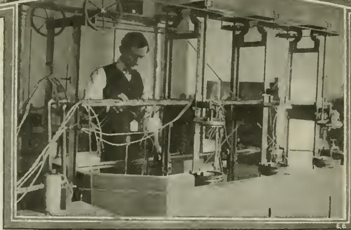
These Men, Experts at the U. S. Bureau of Mines, Do Nothing But Play With Coal. The Calorimeters Above Are Used to Gage the Heat Value of Coal in B. T. U.
