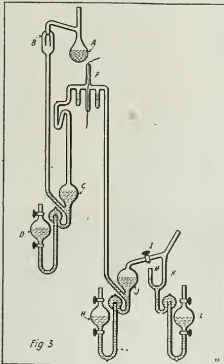
Elaborate Glass Apparatus Used in Order to Fill the Small Capillary Treatment Tubes with the "Radium Emanation". The Bulb "A" Contains the Radium Salt Dissolved in Water, from Which the Gaseous Emanation is Set Free.
