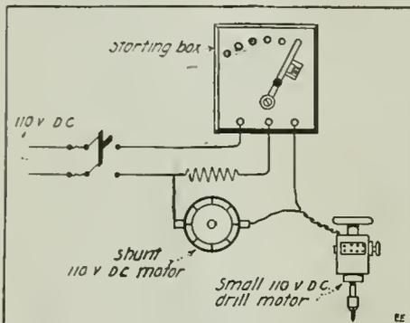
Special Hook-Up for Two 110 Volt D. C. Motors Connected In Series
