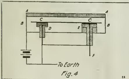
Simplified View of Electrical Method Used in Determining Accurately the Quantity of the Radio-Active Substance in an Applicator. It is Used in Conjunction with a Sensitive Electrometer.
