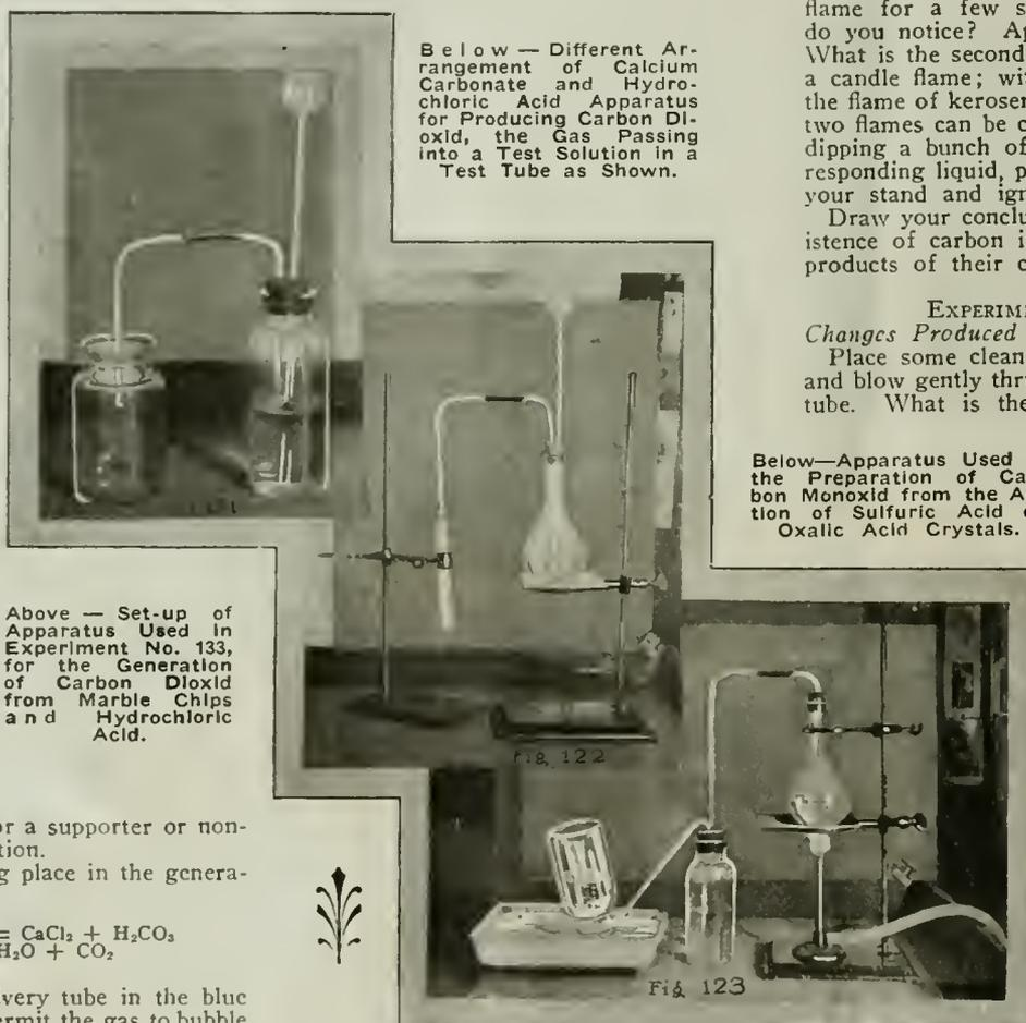
Below — Different Arrangement of Calcium Carbonate and Hydrochloric Acid Apparatus for Producing Carbon Dioxid, the Gas Passing into a Test Solution in a Test Tube as Shown.
