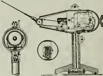
shell-like housing illustrated herewith. A novel driving means is very cleverly worked out, the electric motor being provided with a worm gear, whereby a pair of oppositely disposed arms fastened to the worm wheel rotate continuously and oscillate the fan blade up and down.
