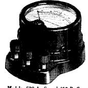
Models 528 A. C. and 489 D. C. Made in high resistance and low resistance models for D. C. service and in double range combinations for A.C. service. This line also includes a triple range—150/8/4 volts for A.C. receiver testing
