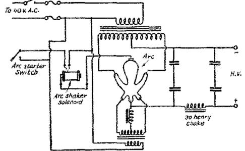
FIG. 2 — THE CONNECTIONS OF THE POWER SUPPLY UNIT
