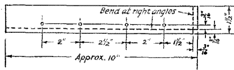
FIG. 1 — THE DIMENSIONS OF THE TEMPLATE FOR LAYING OUT THE POSITION OF THE HOLES ARE GIVEN ABOVE
