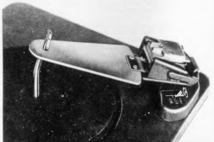
FIGURE 7. SPECIAL RECORD-SHELF GAUGE, SHOWN IN CORRECT POSITION
